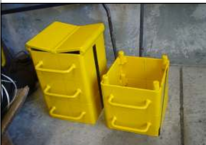
Work stands three blocks high with solid profiled top.
