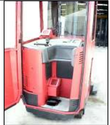
Blower can be seen in the foot well
